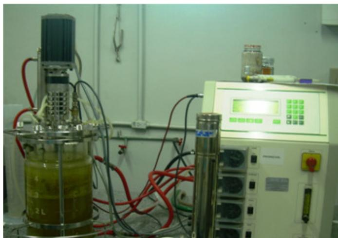
**Figura 5** - Biorreator instrumentado tipo Biostat Braun Biotech International 4,0 L.
