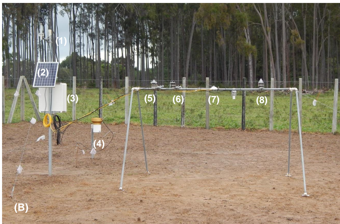
a) 1 – Termohigrometro; 2 - painel solar; 3 - datalogger; 4 - LI200X; 5 - CNR4; 6 - SP-Lite; 7 - CS300. (b) 1- anemômetro; 2 - painel solar; 3 - datalogger; 4 - pluviômetro; 5 - SP-Lite; 6 - CS300; 7 - CNR4; 8 - LP02.
